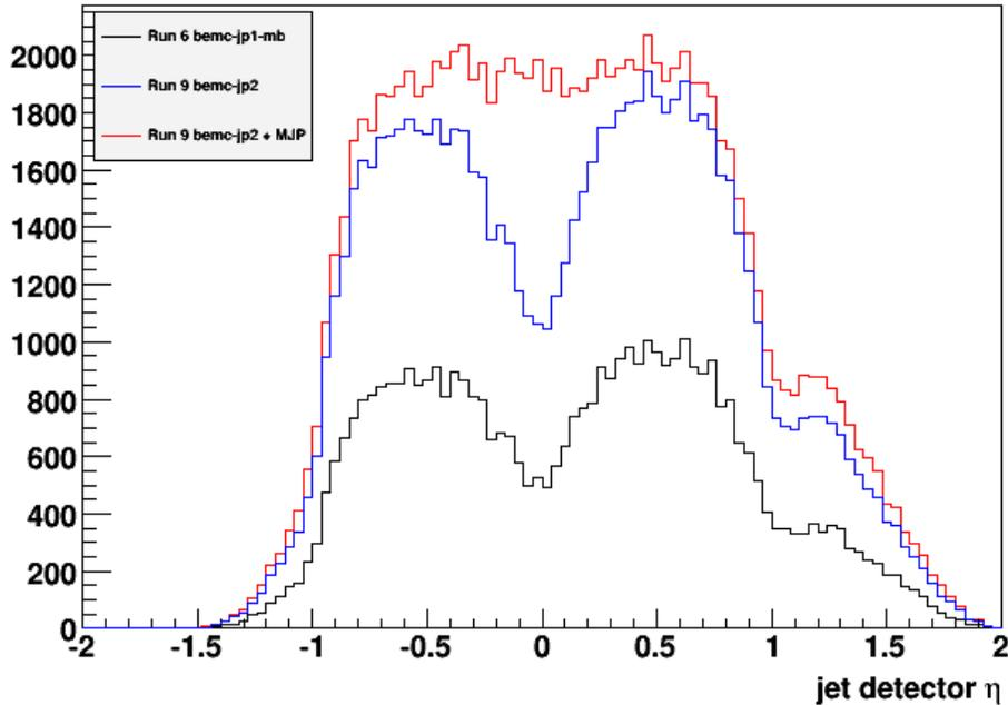
FIG. 1. Impact of the new overlapping jet patch near  $\eta=0$ . The red (blue) curve shows the jet yield for GEANT simulations of 200 GeV p+p PYTHIA events with partonic  $p_T$  in the range 11-15 GeV with (without) the new JP.
